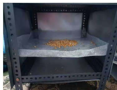
Figure 2. Corn Seed Dryer Frame Using Heating Element with ESP-32 Cam.
